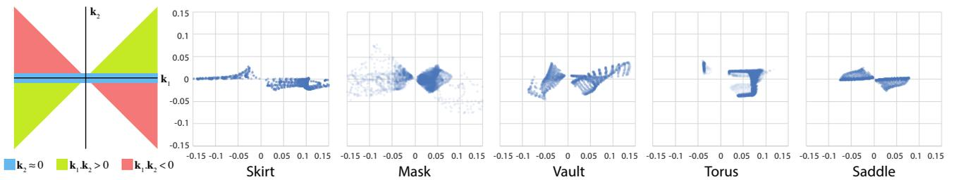
**Figure 10:** Visualization of the two principal curvature values sampled over some of our target surfaces. While we expect our method to be most effective at controlling extrinsic curvature where the target shape is nearly-developable ( $k_2 \approx 0$ , such as throughout the Skirt), most of the surfaces we reproduced also exhibit positive and negative Gaussian curvature (Mask, Vault and Torus), or even solely negative Gaussian curvature (Octopus Saddle).
