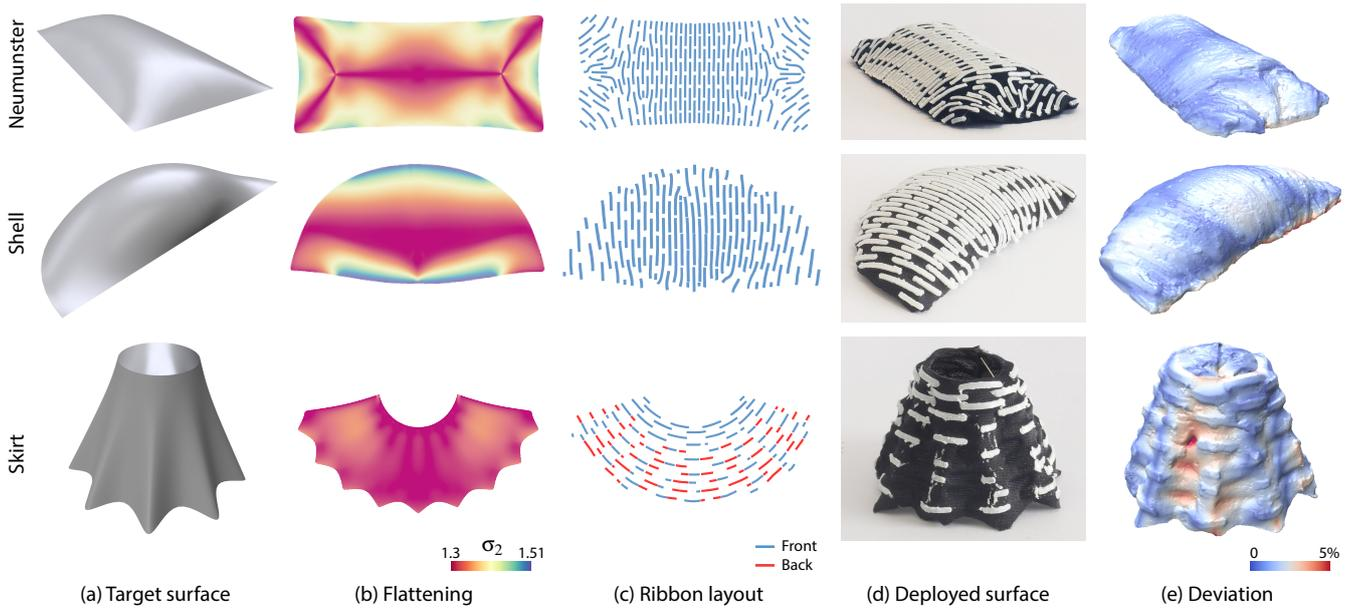
**Figure 9:** Representative results produced with our method, including freeform doubly-curved surfaces (Neumunster and Shell) and a nearly-developable surface achieved by printing on both sides of the fabric (Skirt). We visualize the deviation of the scanned fabricated shape from the target surface, expressed as percentages of the bounding box diagonal of the target.
