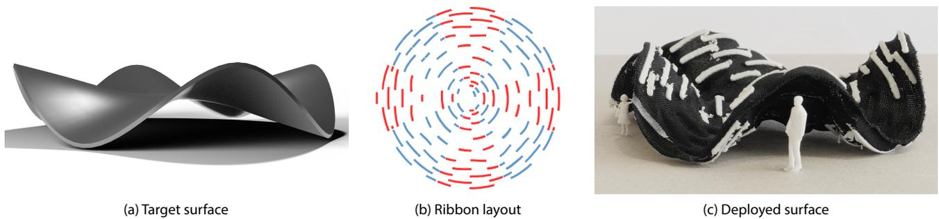
**Figure 1:** Given a target 3D surface (a), our method computes a flat layout of plastic ribbons (b) which, when printed on pre-stretched fabric, causes the surface to deploy into 3D when the fabric is released (c). We designed a custom frame to easily print ribbons on both sides of the fabric (b, red and blue), allowing us to reproduce surfaces with positive and negative extrinsic curvature.
