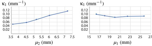
**Figure 5:** The curvature  $\kappa_1$  of our metamaterial varies not only as a function of plastic thickness  $\tau$ , but also as a function of spacing  $\mu_2$  in the transverse direction (left, with  $\mu_1 = 22.5$ mm and  $\tau = 0.5$ mm). In contrast, varying spacing  $\mu_1$  in the ribbon direction has little impact (right, with  $\mu_2 = 6$ mm).
