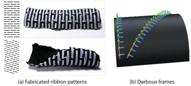
**Figure 3:** Due to the bilayer effect, parallel plastic ribbons roll to form a cylinder (a, top). Attempting to orient the ribbons away from the direction of maximum curvature still yields a cylinder as ribbons resist torsion (a, bottom). On a curved surface, curvature lines are the only curves with zero geodesic torsion, as visualized by sliding a Darboux frame along the curve and observing its rotation around the curve tangent (b, after [IBB15]).
