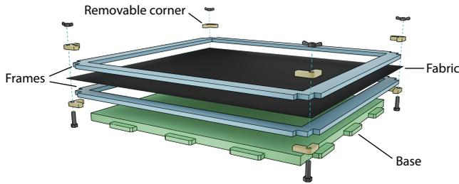
**Figure 8:** Our frame structure is composed of two rigid frames, in between which the fabric is clamped in tension. These frames sit on a base that attaches to the printer bed. The four corners of the frames can be removed to be fixed to the sheet of fabric before stretching.
