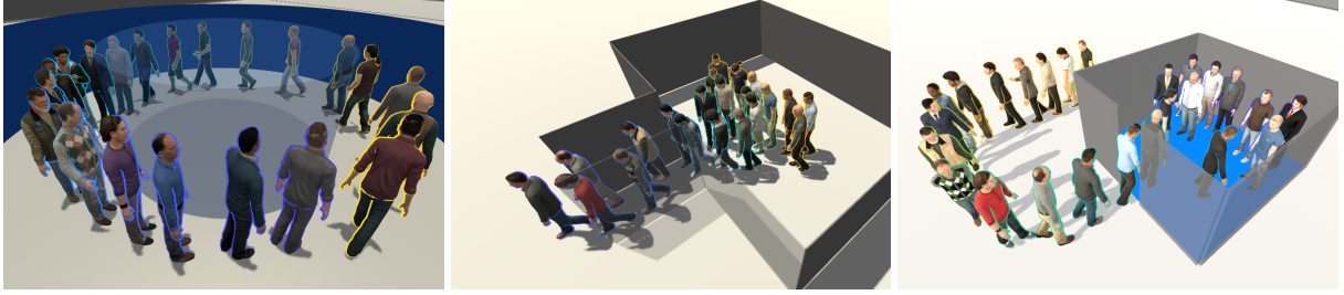
Fig. 1. Snapshot of crowd motions generated using the one-man-crowd approach. A single user successively embodies each displayed virtual agent in the order indicated by the highlighting colour (from blue to yellow). We studied 3 scenarios that replicated existing experiments from left to right: circular unidirectional flow, bottleneck situation, inflow behaviour (entering a lift).
