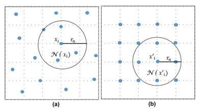
**Fig. 1** Illustration of an RGG (a) and a (DGG) (b) for n = 16
