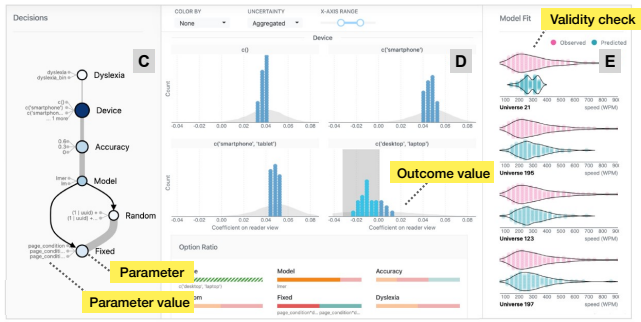
Figure 15: Screenshot of the Boba system [LKAH20]. Panel C shows the design space of parameters and their relationships; parameters that are source of sensitivity are in a darker color. Panel D is a trellis of dotplots of outcome values, subsetted by parameter values. Panel E shows predictive distributions from each universe compared to the observed data.
