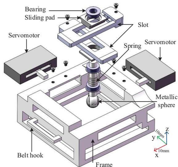
Fig. 1. Assembly of the 2-DoF wearable cutaneous device. A metallic sphere either provides position/location feedback or skin stretch in a  $12 \times 12$  mm workspace. We tested the device at the forehead, forearm, and hand. A video is available as supplemental material and at <https://youtu.be/38BHsYQC6uM>.
