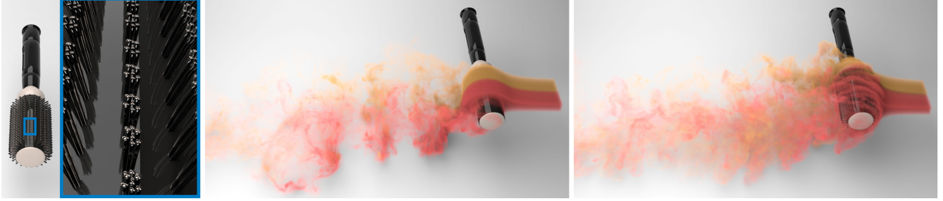
Fig. 4. Hair brush. The translating and rotating motion of a hair brush containing hundreds of bristles (left) creates fine vortices in its wake as well as around the bristles (right) as evidenced by the evolution of the smoke passing around it, properly capturing the intricate fluid-solid interaction engendered by this complex geometry. Compared to the coupling with bristles (right), the smoke near the hair brush without bristles (middle) is much smoother, and the wake flows contain relatively large vortices, indicating the efficacy of subgrid approximation in handling such complex solid shapes.
