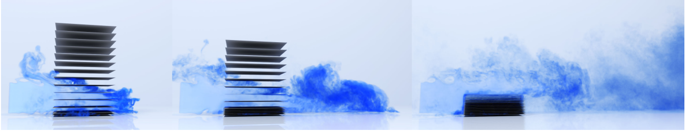
Fig. 13. Smoke flow through stacked plates. Smoke is blown towards a falling stack of thin plates. While smoke freely flows between separate plates, they become an airtight obstacle when they are stacked on top of each other. Our boundary treatment based on subgrid approximation deals with both cases seamlessly: plates getting closer accelerate the flow in between them, while tightly stacked plates are treated as thick solids.
