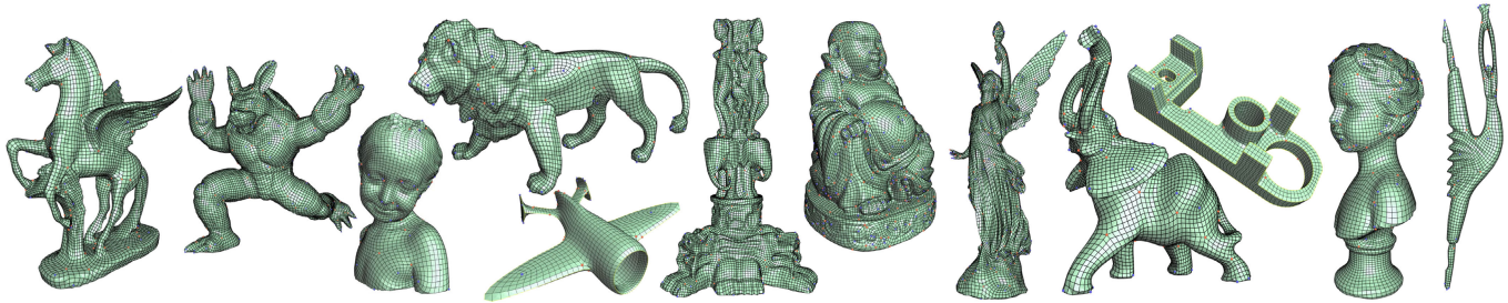
Fig. 22. Zoo. Examples of quad meshes from [Fang et al. 2018], of various sizes, on which a few automatic Q-zip batches were performed based on the heuristic for connectivity optimization described in Sec. 4.1. Irregular vertices are marked as colored balls, and yellow lines indicate sharp features.
