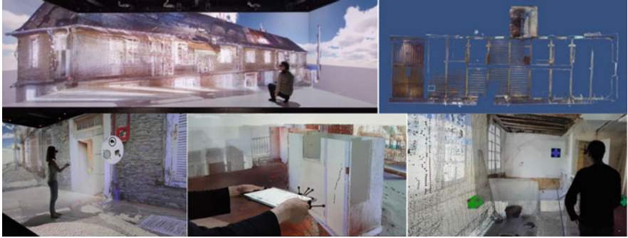
Fig. 48.12 Immersive visualization of the point cloud at 1:1 (top, left), example of 2D cut view obtained with the tool (top, right), interactions with the point cloud in high definition (bottom, left), cutting plan manipulation with a tracked tactile tablet (bottom, center), and position of a photographic view in the Virtual Reality application (bottom, right)
