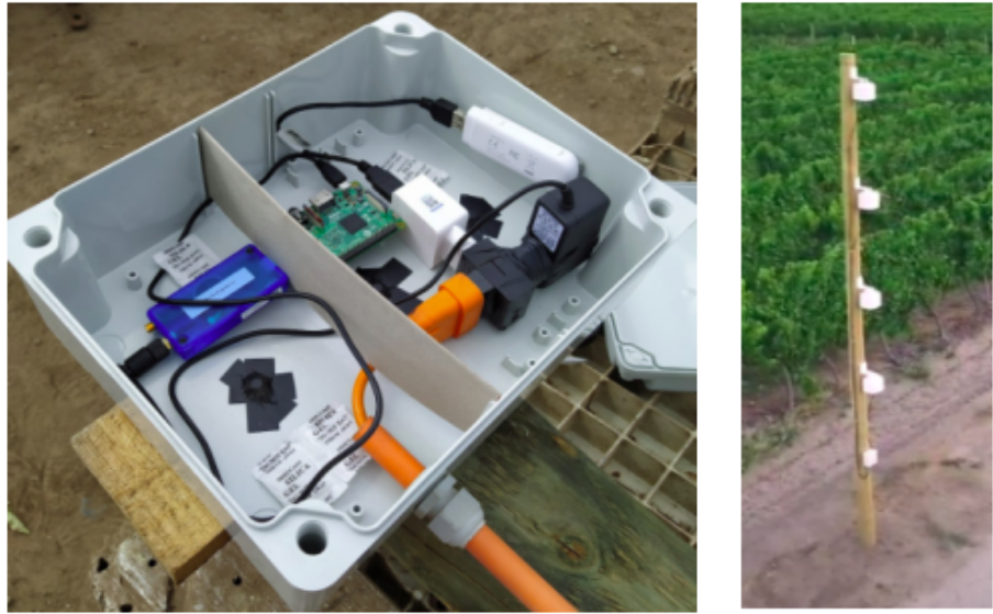
Figure 2. IoT platform installed on the experimental field composed by temperature and humidity sensors.
