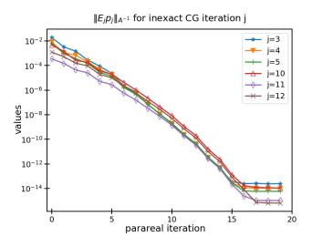
Figure 3: Profile of  $\|\mathbf{E}_{j}\mathbf{p}_{j}\|_{\mathbf{A}^{-1}}$  for different CG iterations
