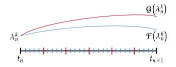
The parareal algorithm proceeds iteratively by computing the solution  $\lambda_{n+1}^k \approx \lambda(t_{n+1})$  at the subintervals for given  $\lambda_n^k$  at time  $t_n$  and iteration k. An initial configuration is obtained by a serial run of the coarse propagator  $\mathcal{G}$  over the whole time domain. Thus,
