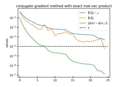
For the same minimisation tolerance now the matrix-vector product is supplied through the Parareal method. To mimic the same results obtained through the exact matrix-vector product we need to choose a very low tolerance for parareal. For  $\epsilon_{\rm p} = 10^{-12}$  as a fixed stopping criterion, it takes 388 parareal iterations.
