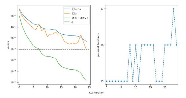
The above 1-D shallow water model with the given parameters is now considered in the context of Data Assimilation problem. From the above exact CG solution with  $\epsilon_{cg} = 10^{-4}$ , we find the value of  $||r_k||_{A^{-1}}$  and use it in (22) to calculate a suitable stopping criteria for the inexact CG. We find that  $\epsilon_{icg} = 1.12 \times 10^{-7}$ .
