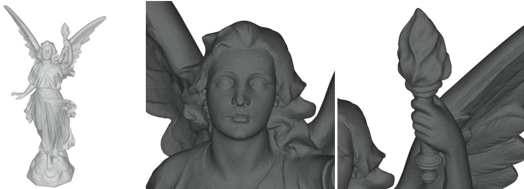
Fig. 2 Rendering of a large mesh of 14M vertices and 28M triangles in 7.5 seconds (total time) on a laptop.
