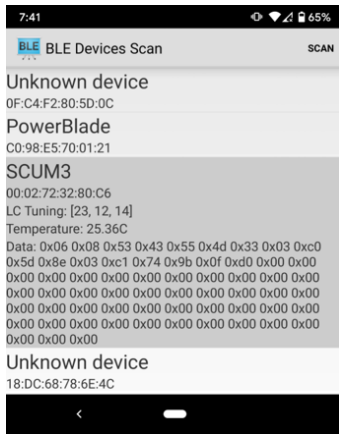
Fig. 4. The BLE sniffer app running on a Google Pixel 2 XL displaying a BLE advertising packet received from a SC \mu M mote while the mote is in a temperature chamber.
