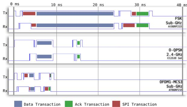
**FIGURE 1.** Timeslot templates for the three PHYs, for a 100 B data payload with acknowledgement. Red markers highlight when SPI transactions between the micro-controller and the AT86RF215 take place. We use a 40 ms timeslot duration for all the PHYs in both multi-PHY and single-PHY architectures (source: [17]).
