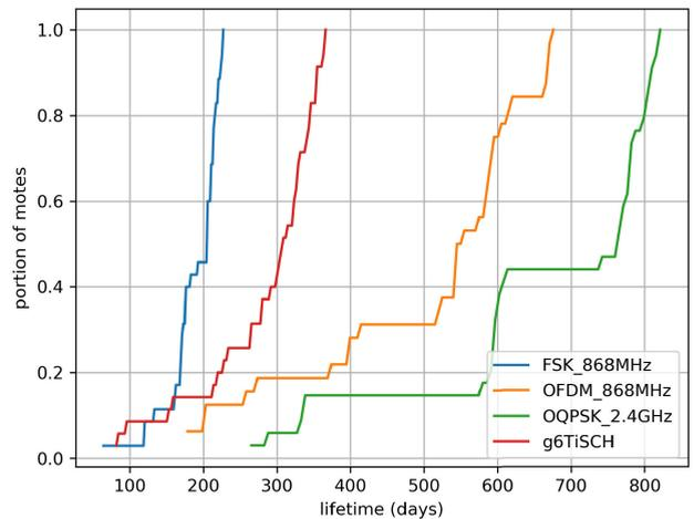
**FIGURE 15.** Cumulative distribution function of battery lifetime in the network demonstrates the g6TiSCH improving the energy footprint of the network compared to a pure long range FSK 868 MHz network.
