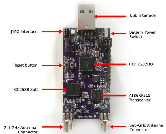
**FIGURE 6.** The OpenMote B board with multi-PHY support.
