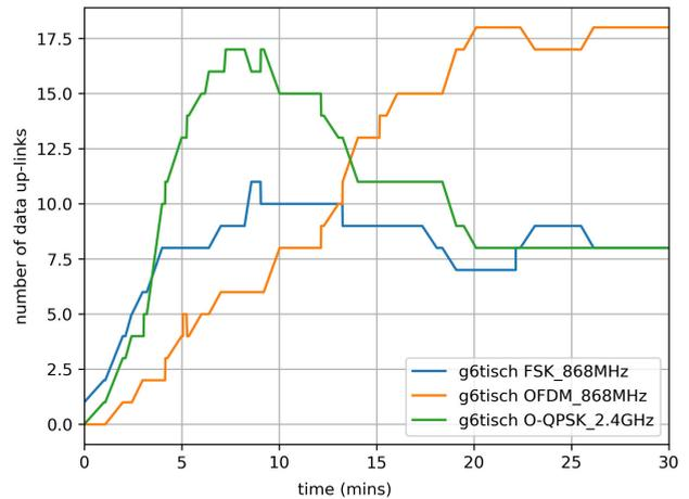
**FIGURE 9.** As the g6TiSCH data collection tree is forming, it routes up-link traffic over diverse PHYs.
