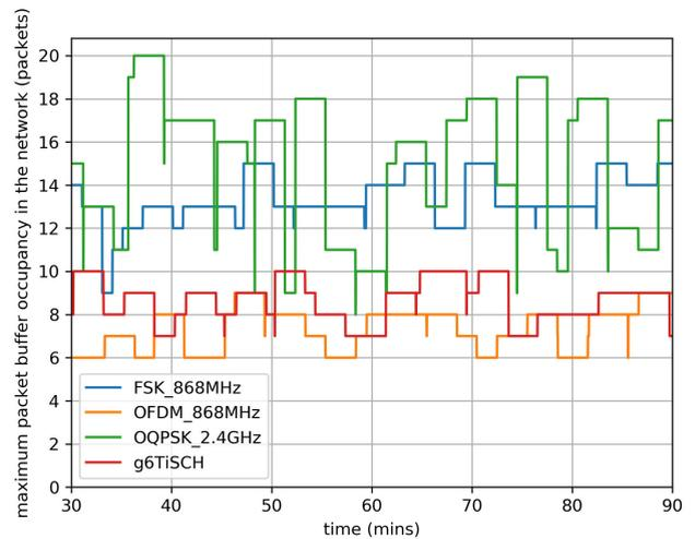
**FIGURE 12.** Improved overall link quality in g6TiSCH leads to efficient buffer usage due to less re-transmissions and forwarding. Packet buffer is efficiently used and packets are not dropped due to buffer overflow.
