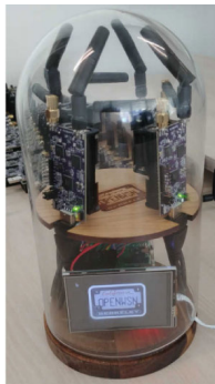
FIGURE 7. The OpenTestbox used for experimental evaluation in the Open Testbed (source: [37]).
