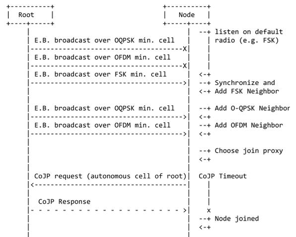
**FIGURE 2.** Neighbor discovery is adapted to listen on different PHYs for new neighbors. Use of hybrid PHYs on minimal cells enable faster neighbor discovery and Constrained Join Protocol handshake. Adapted from IETF draft [36].
