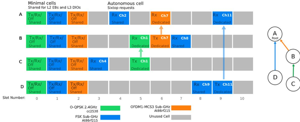
**FIGURE 4.** Example of a multi-PHY slot frame in the resulting generalized 6TiSCH architecture. A minimal cell for each PHY-layer enables discovery of different radios. FSK 868 MHz is used for autonomous cells. Node C allocates dedicated O-QPSK 2.4 GHz cells for its parent B. Node B allocates dedicated OFDM 868 MHz cells for its parent A. Node C allocates dedicated FSK 868 MHz cells for its parent A.
