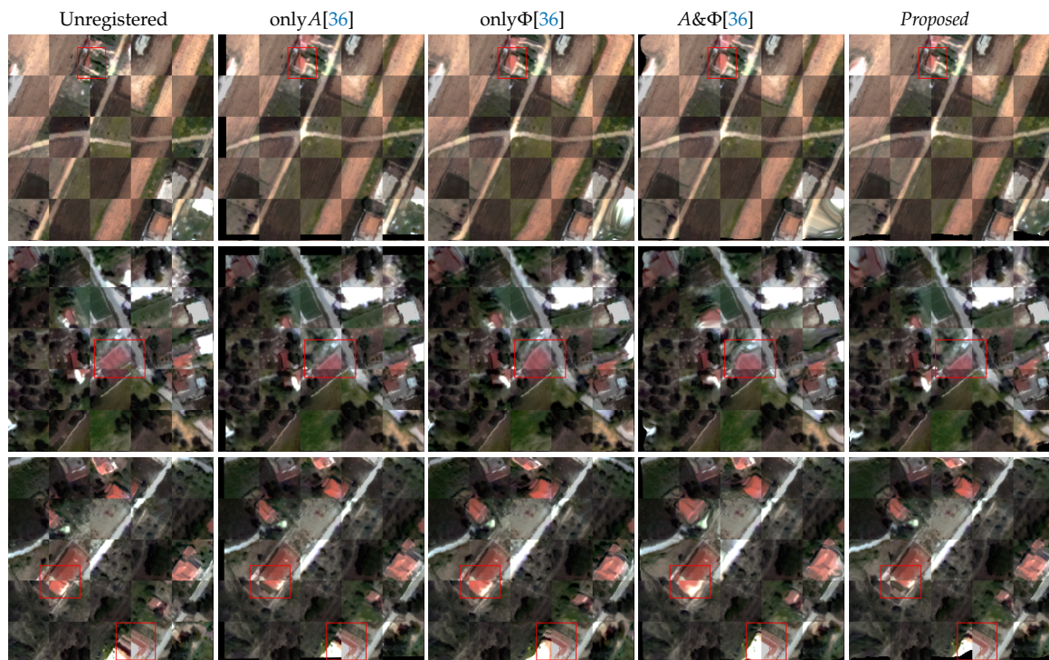
Figure 4. Qualitative evaluation on different pairs from the Attica VHR testing regions. Different approaches from [36] are compared i.e., from left to right: Unregistered raw data, results: only A , only \Phi , A & \Phi , Proposed.
