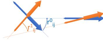
Fig. 6: Non orthogonal frame fields have two angular differences  $r_{ij}^0$  and  $r_{ij}^1$ , one for each pair of vectors.
