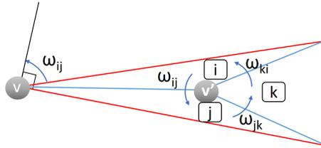
Fig. 8: Local fix of a sharp corner: We set  $\omega_{ij} \leftarrow \theta_v - \pi/2$  to force  $I(v) = 1/4$ . If  $\omega_{jk}$  and  $\omega_{ki}$  are null, then  $d\omega(v') = \theta_v - \pi/2$ . Therefore, the final frame field will have  $r_{ij} = \omega_{ij}$ ,  $r_{jk} = r_{ki} = \theta_v/2$ , leading to an index 1/4 at  $v'$ .
