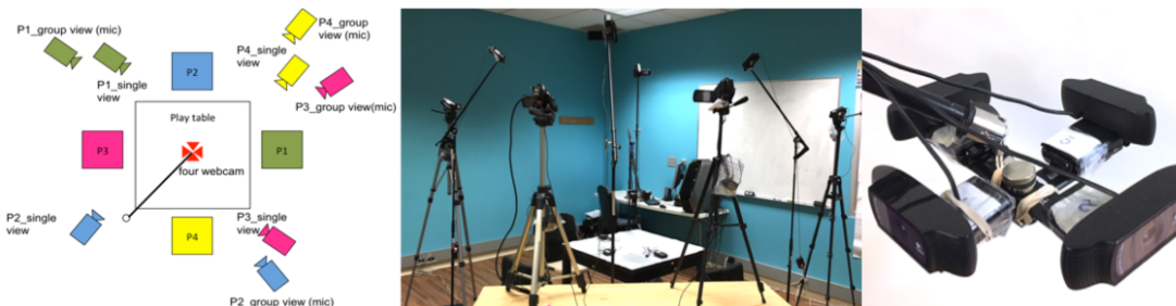
Fig. 2. In-lab study data collection apparatus. Left: equipment arrangement; Middle: real arrangement; Right: fixture of four Webcam devices.
