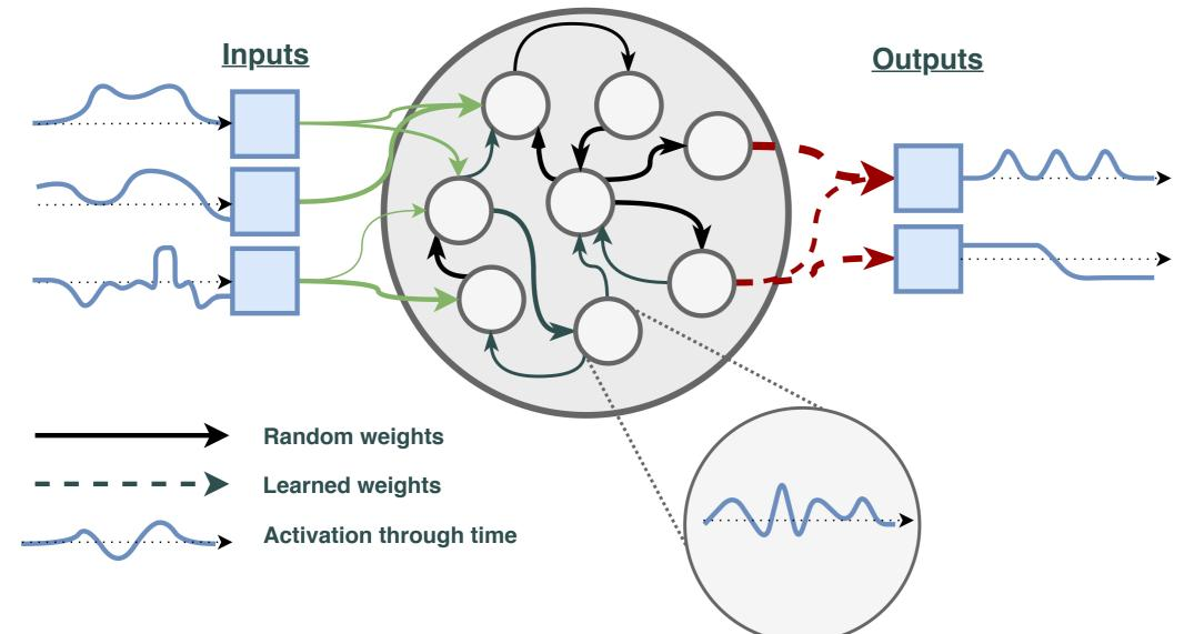
Figure 1: Echo State Networks are an instance of the Reservoir Computing paradigm using units with continuous states
