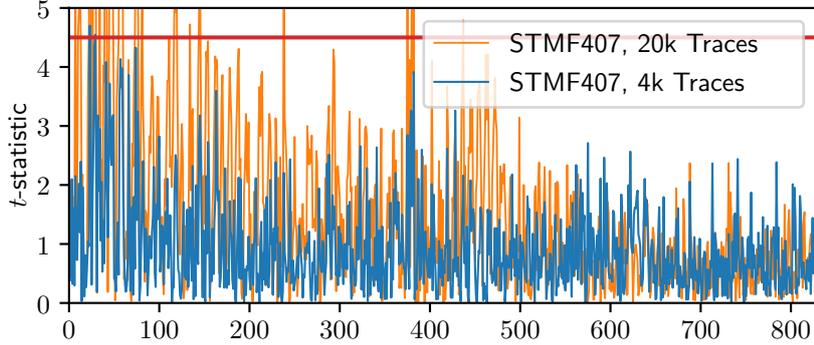
Figure 7: Physical leakage is detected when the optimized 1<sup>st</sup> order PRESENT S-Box is executed on an Arm Cortex M4F microcontroller despite being secure in our model for CM0+ and leakage free on two CM0+ microcontrollers. The  $x$  axis represents sample points.
