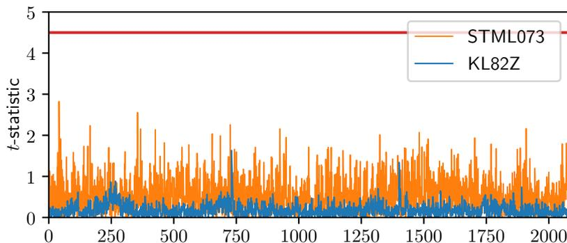
Figure 6: Physical leakage detection  $t$ -statistics of optimized 1<sup>st</sup> order PRESENT S-Box assessment,  $x$  axis represents sample points.
