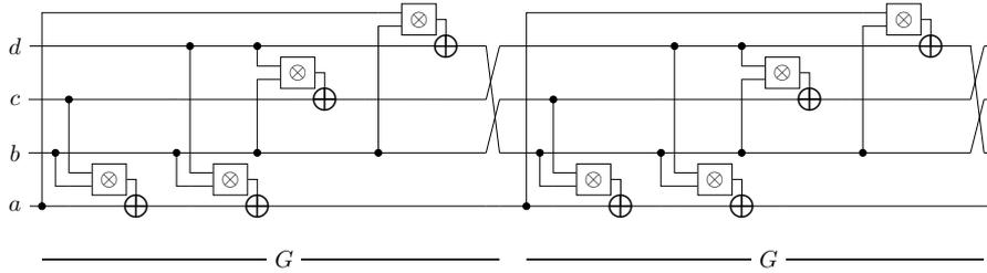
Figure 5: The Non-Linear Layer of the Present S-Box
