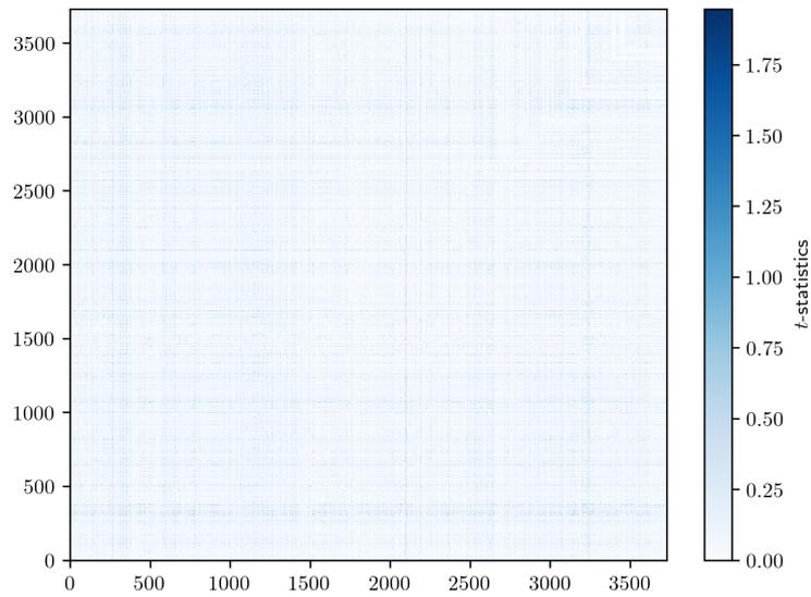
Figure 8: Bivariate TVLA of the optimized 2<sup>nd</sup> order PRESENT S-Box executed on the KL82Z microcontroller. No significant leakage is detected for every pair of sample points on the  $x$  and  $y$  axis as the values are far below the threshold of 4.5.
