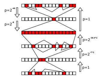
Fig. 3. Classical boomerang attack on SAFER++ (Fig. 4 in [3])
