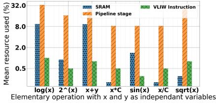
Fig. 5: Pipeline resources used by each elementary operation.
