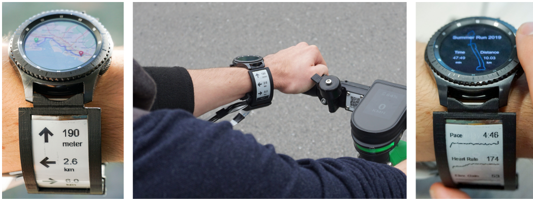
Figure 5.4: Smartwatch with additional displays embedded in the straps [37]; a person can glance at these displays without additional movements or interactions. Images © 2020 Tom Horak and Konstantin Klamka.
