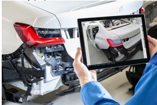
Fig. 11. A video see-through method for inspection of parts after assembling (source: [22]).
