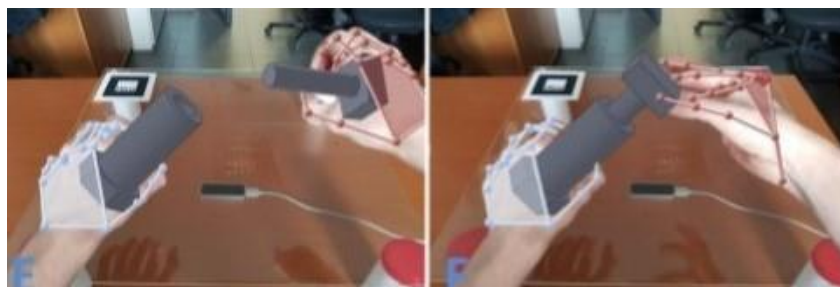
Fig. 16. Sequence of virtual assembly by augmented reality (source: [30]).
