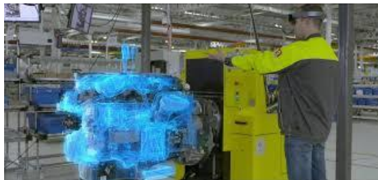
Fig. 12. Microsoft HoloLens smartglasses used for quality control of Renault Trucks engines (source: [23]).
