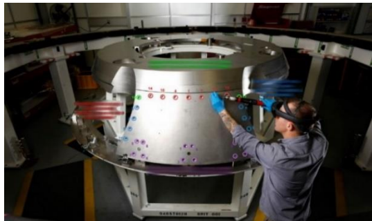
Fig. 8. Head-mounted display used at NASA for assembling spacecraft parts (source: [17]).
