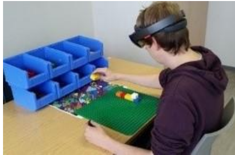
Fig. 2. HMD used to support simple assembly tasks of LEGO® bricks (source: [7]).
