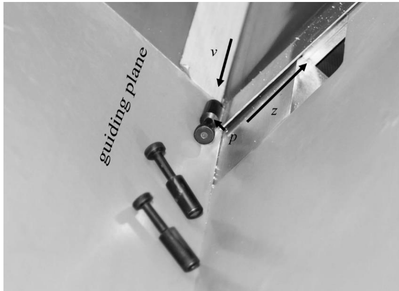
Fig. 4. Orientation process of exemplary workpieces with the parameters v (conveyor), p (nozzle) and z (linear positioning)
