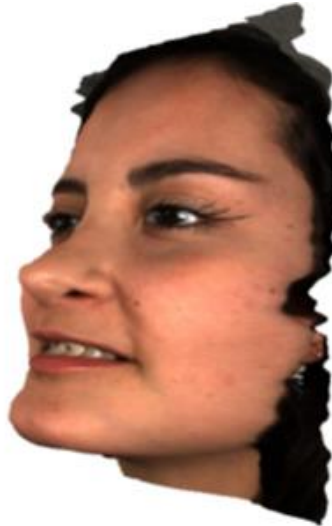
Fig. 9. Real-time 3D image as obtained by Raytrix light field camera.
