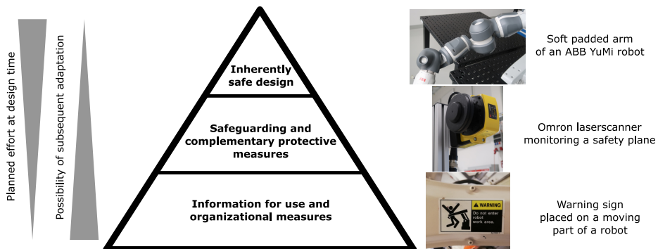
Fig. 1. Measures to reduce risk according to ISO 12100 and a selected example
