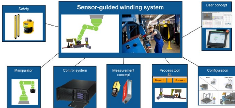
Fig. 4. Structure and components of a sensitive robot system
