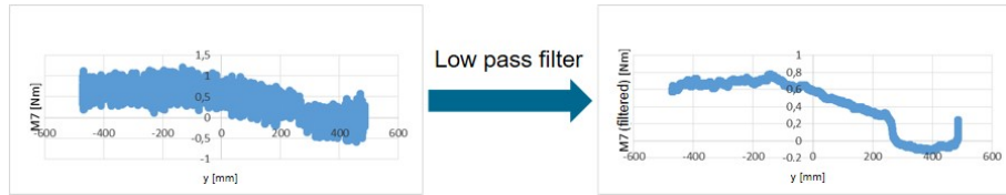
Fig. 11. Integration of the low-pass filter to smooth the measured curve of the torque
