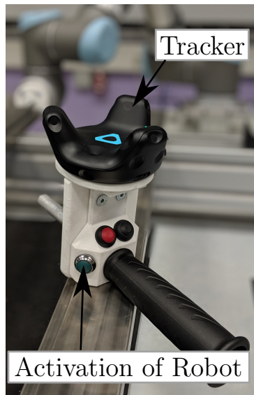
Fig. 3. Worker tool with tracker.
