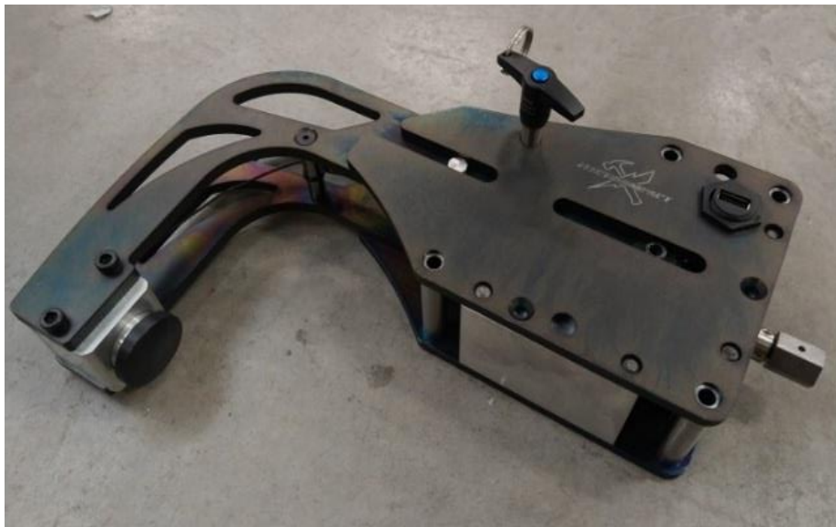
Fig. 17. Manual Panel Clamp with Load Cell Feedback
