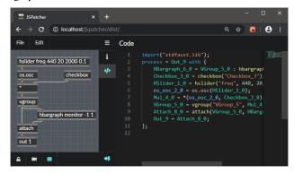
Figure 13 The generated code can be previewed in on the right panel (synchronized to the patcher)
