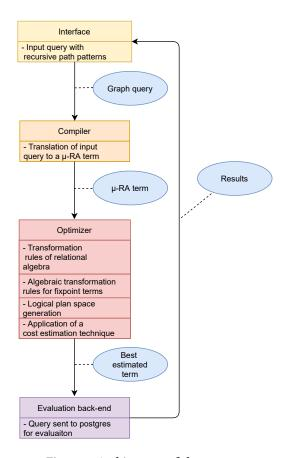
Figure 1: Architecture of the system.
