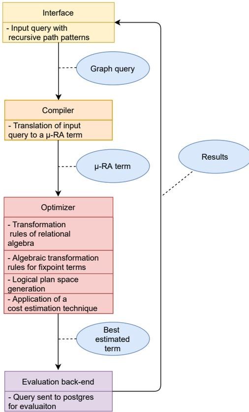
Figure 1: Architecture of the system.
