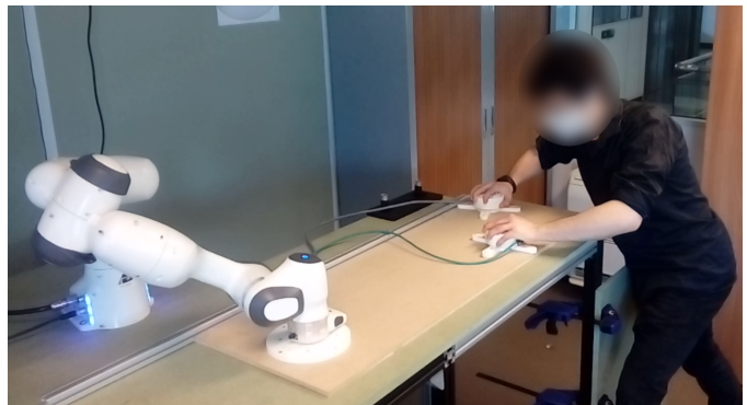
Fig. 1. Subject performing an experiment of a milling task in carpentry using a physically realistic mock-up. The wooden part is being pushed through handles incorporating 6-axis F/T sensors. A 7-DOF collaborative robot is attached to the wooden part and reproduces the cutting forces based on a wood cutting model
