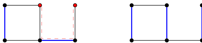
Figure 1.1: Example of an M -augmenting path. In the figure to the left, there is a matching M of two blue edges, the two red vertices are unmatched, and there is an M -augmenting path P (dashed red) between these two unmatched vertices. We obtain a new matching with one more edge by removing blue edges in P from M and adding the other black edges in P to M . We then get the matching depicted in blue on the figure to the right.
