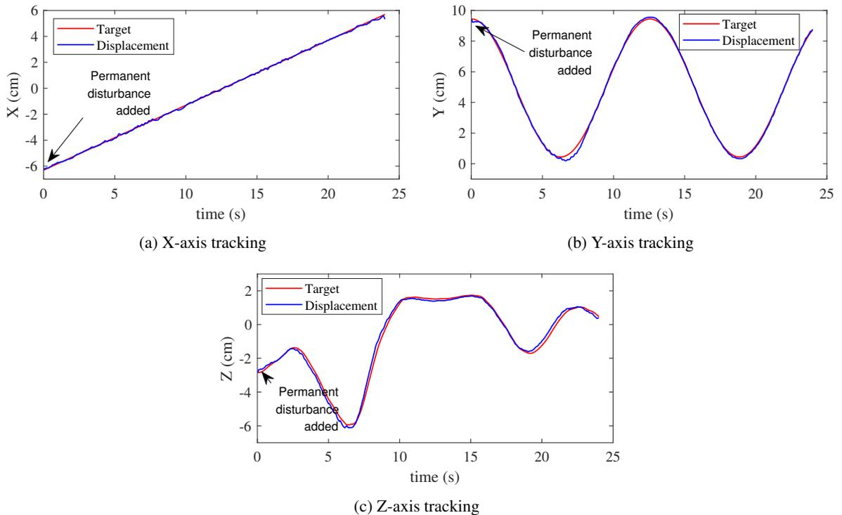
**Figure 11:** Permanent disturbance test using the proposed controller
