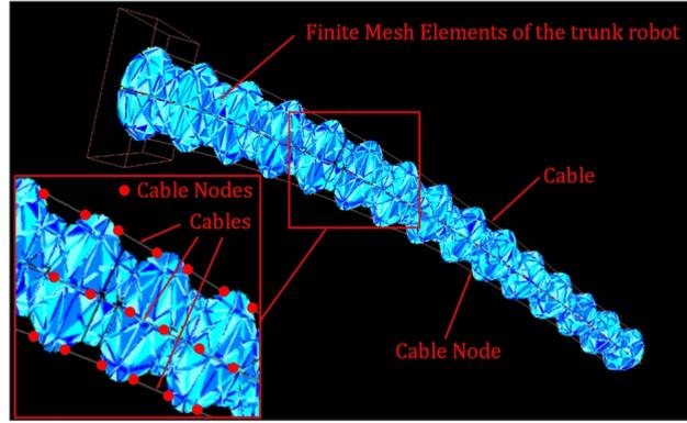
**Figure 2:** Mesh elements of the modeled trunk robot.
