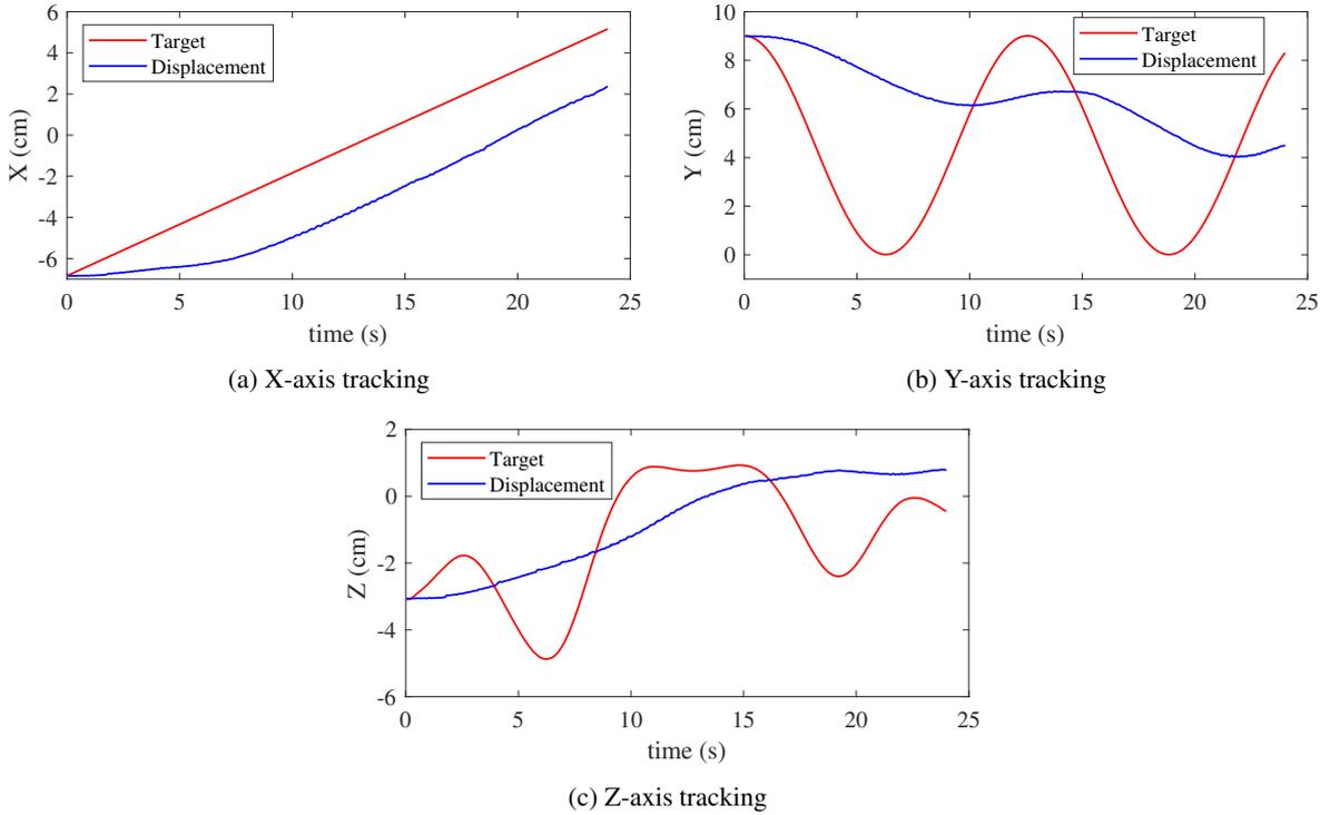
**Figure 7:** Trajectory tracking using a common PID controller
