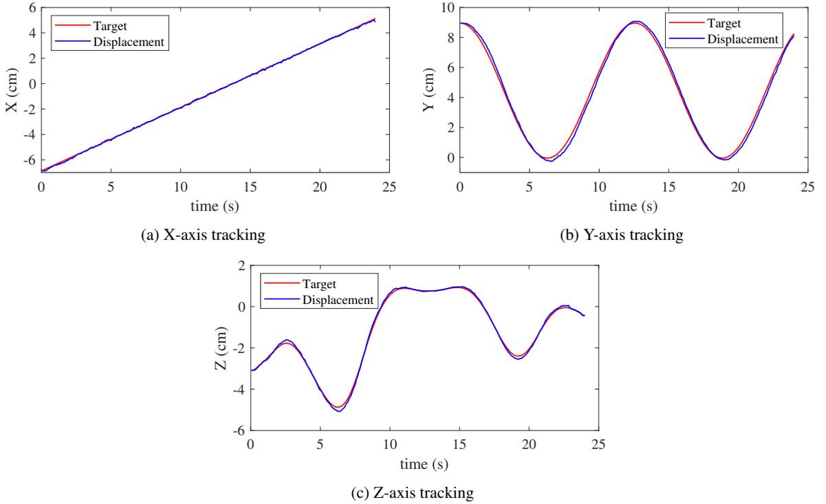
**Figure 8:** Trajectory tracking using the proposed controller
