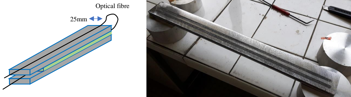
Figure 2. Position of the optical fibre and example of optical fibre application on specimen
