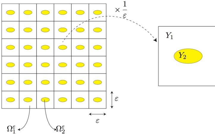
Fig. 1 – The composite periodic material and the corresponding reference cell  $Y$  ( $d = 2$ ).
