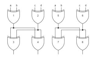
**Fig. 2.** An example of a small differential Public Physical Unclonable Function (dP-PUF). Left (1-4) and right (5-8) circuits are the same in functionality. The challenge (abcd) is presented at both sides at the same time. However, the output of gates 3-4 and 7-8 stabilizes at different times due to manufacturing variability. The fastest propagating signals determine the corresponding response that forms the CRP.
