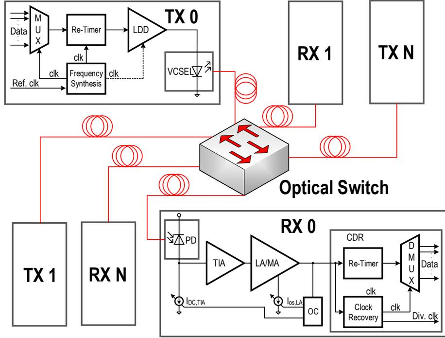
Fig. 1: Optical communication link in a network.
