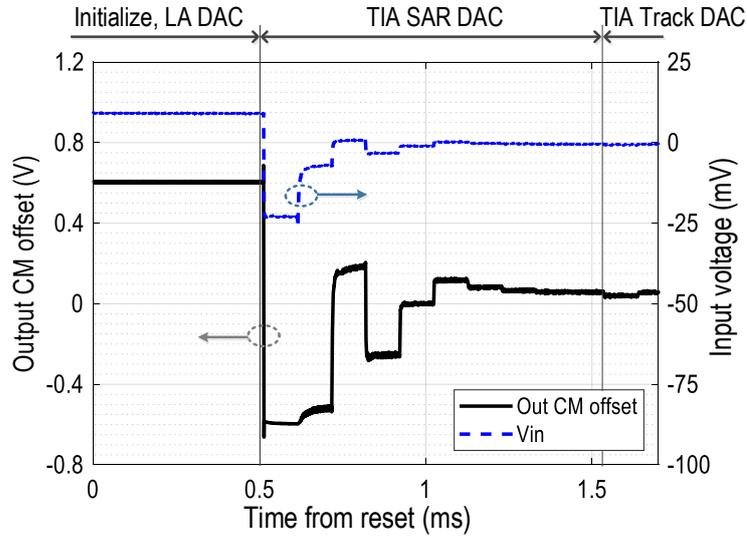
Fig. 14: Oscillogram of the MS OC, output CM offset and input signal.
