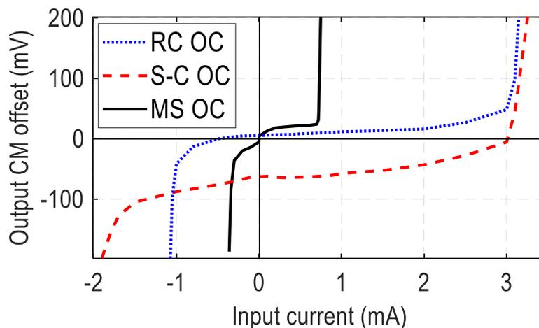
Fig. 17: Measured dynamic range of the OC architectures.
