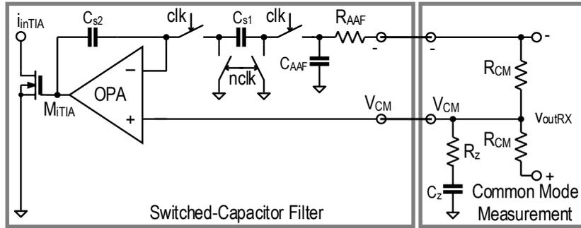
Fig. 7: Conventional S-C low-pass filter based offset compensation schematic.
