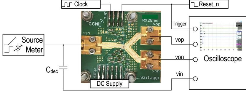
Fig. 13: Measurement setup.
