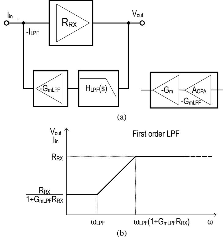
Fig. 4: Lower cut-off frequency  $f_{LCO}$  (a) System view and (b) calculation for a first order LPF.
