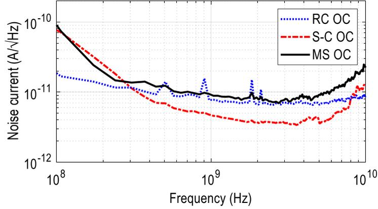
Fig. 18: Measurement of the input referred noise current.
