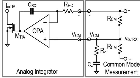
Fig. 6: Conventional RC low-pass filter based offset compensation schematic.
