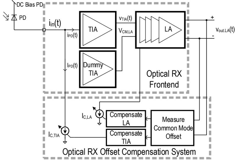
Fig. 2: Offset compensation system in an optical RX frontend.
