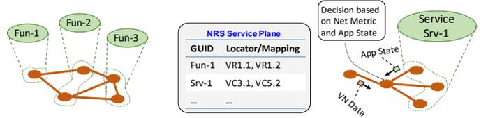
Fig. 4. Application Specific Advanced Routing in NOVN
