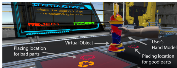
Fig. 5. Users face a table onto which a virtual part is extruded. They can pick it up and inspect it, then they select whether the part is flawed or good. This explicitly indicates their future to place the part either into the disposal bin or onto the conveyor belt. The robot drives to the chosen release position to preempt the user's release of the part, after which it removes the tangible object from the interaction space as the virtual part is either destroyed or removed from the scene.
