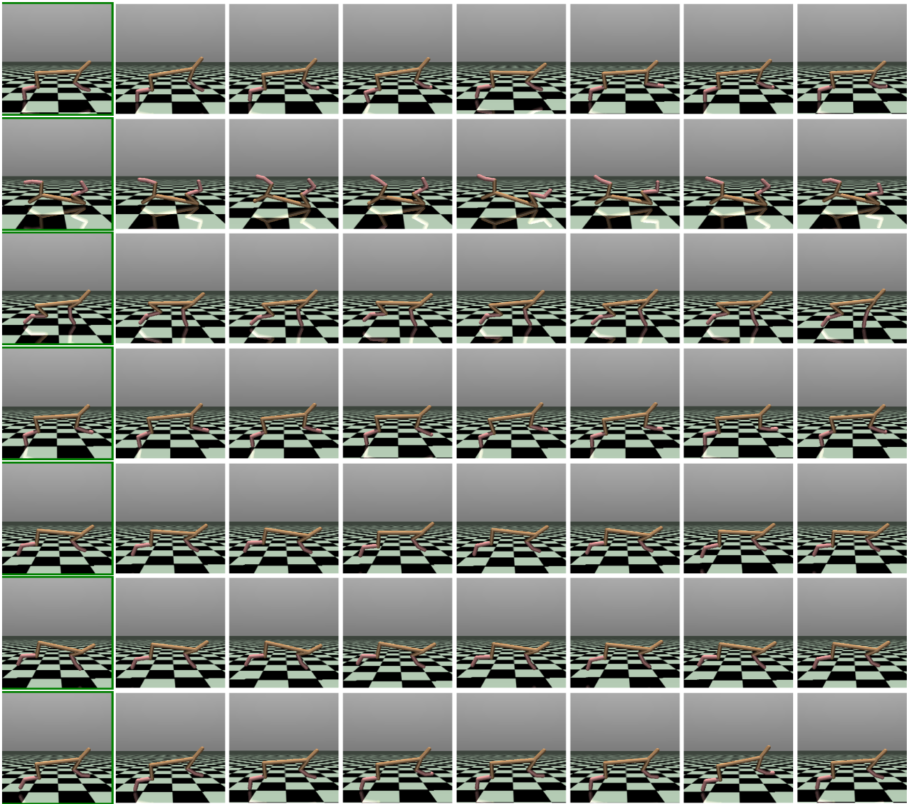
Figure 6. State similarity learned by PLOFF for HalfCheetah on the medium-replay dataset. For each row, the leftmost image is the state for which we compute nearest neighbors in the dataset \mathcal{D} for the metric induced by \Psi (ranked by decreasing level of similarity).
