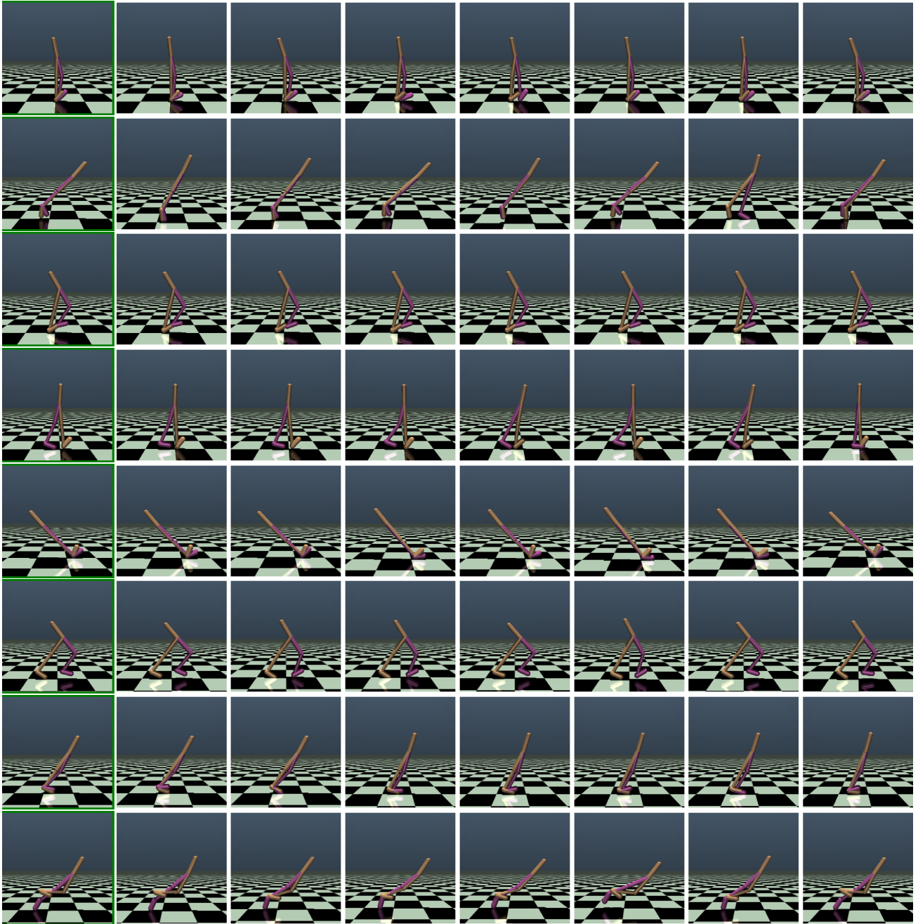
Figure 8. State similarity learned by PLOFF for Walker2d on the medium-replay dataset. For each row, the leftmost image is the state for which we compute nearest neighbors in the dataset \mathcal{D} for the metric induced by \Psi (ranked by decreasing level of similarity).
