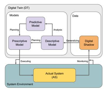
Fig. 1: Conceptual framework for DTs based on MODA [3]
