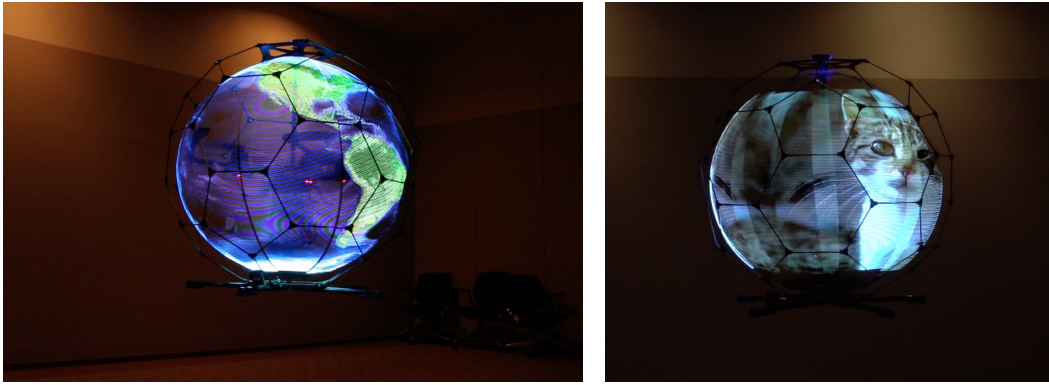
Figure 1.12: A more advanced version of the iSphere [45] with an effective display resolution of 760 \times 320 pixels. Images © 2020 NTT Docomo, used with permission from Wataru Yamada.
