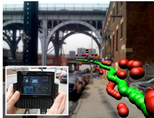
Figure 4.12: SiteLens: Non-stereoscopic display of air quality measurements (non-volumetric, geo-spatially anchored data) using 3D representations in an outdoor environment [94]. Image © Sean White, used with permission.
