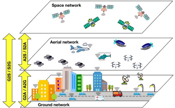
Fig. 2: Integrated space-air-ground network in 6G scenarios.
