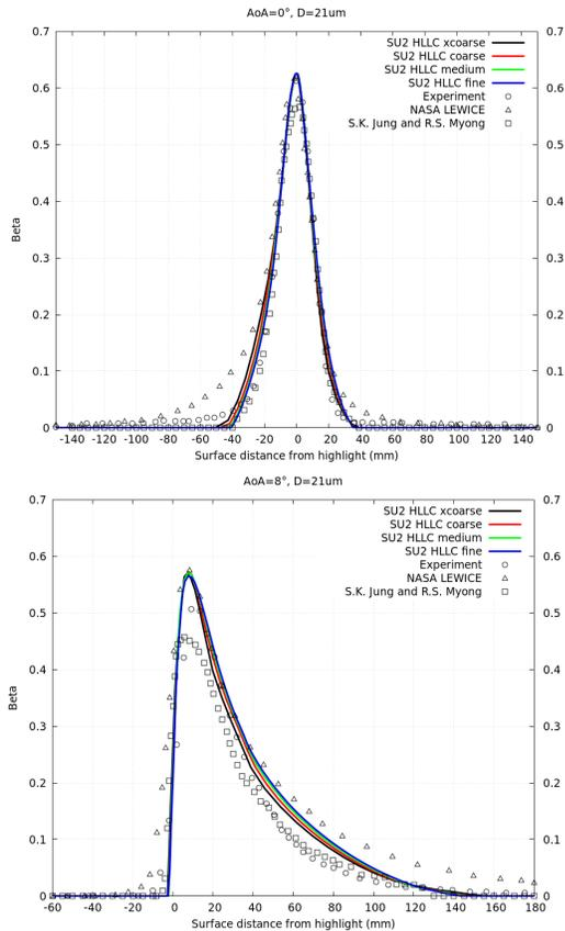
Figure 5: Local collection efficiency sensibility to the mesh size on a NACA 65<sub>2</sub>415 airfoil,  $d = 21 \mu\text{m}$ , Mach=0.23, AoA=0° and AoA=8°, chord=0.928m
