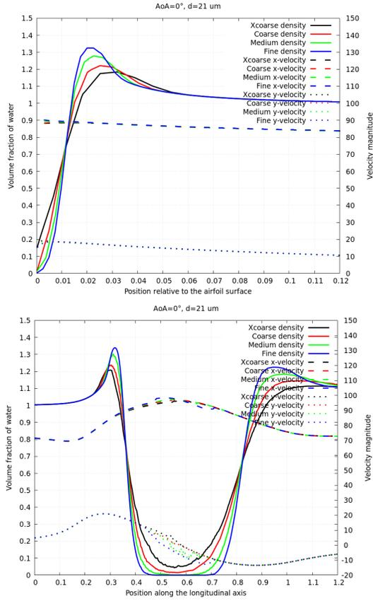
Figure 7: Normal and tangential volume fraction of water and velocity on the NACA 65<sub>2</sub>415 airfoil,  $d = 21 \mu\text{m}$ , Mach=0.23, AoA=0°, chord=0.928m
