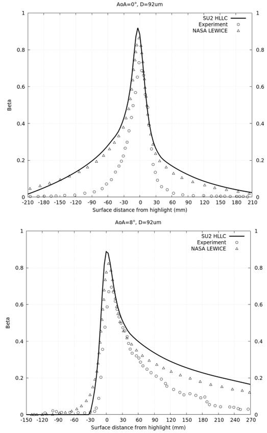
Figure 10: Local collection efficiency on a NACA 65<sub>2</sub>415 airfoil,  $d = 92 \mu\text{m}$ ,  $\text{Mach}=0.23$ ,  $\text{AoA}=0^\circ$  and  $\text{AoA}=8^\circ$ ,  $\text{chord}=0.928\text{m}$
