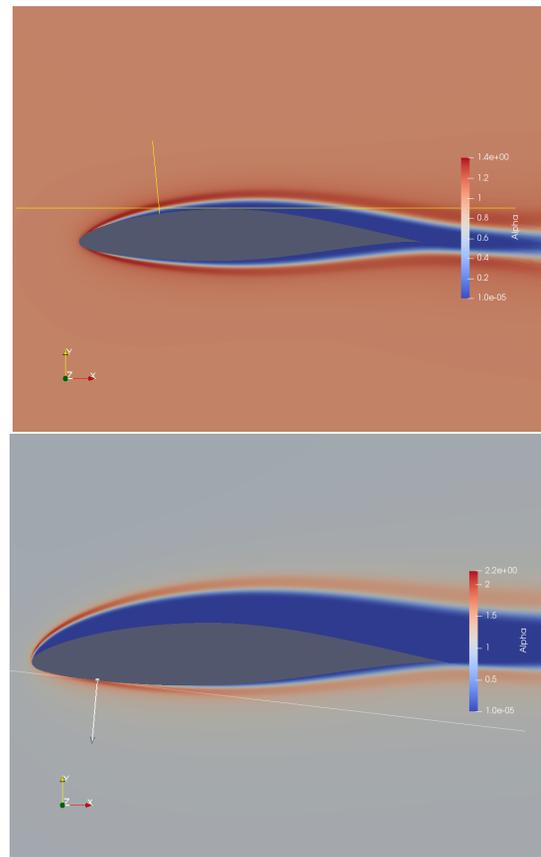
Figure 6: Cutting lines on the NACA 65<sub>2</sub>415 airfoil,  $d = 21 \mu\text{m}$ , Mach=0.23, AoA=0° and AoA=8°, chord=0.928m
