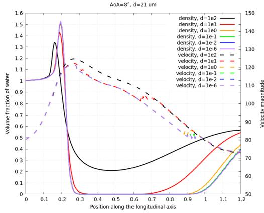
Figure 9: Tangential volume fraction of water and velocity for different stabilisation parameters on the NACA 65<sub>2</sub>415 airfoil on the upper surface,  $d = 21 \mu\text{m}$ ,  $\text{Mach}=0.23$ ,  $\text{AoA}=8^\circ$ ,  $\text{chord}=0.928\text{m}$
