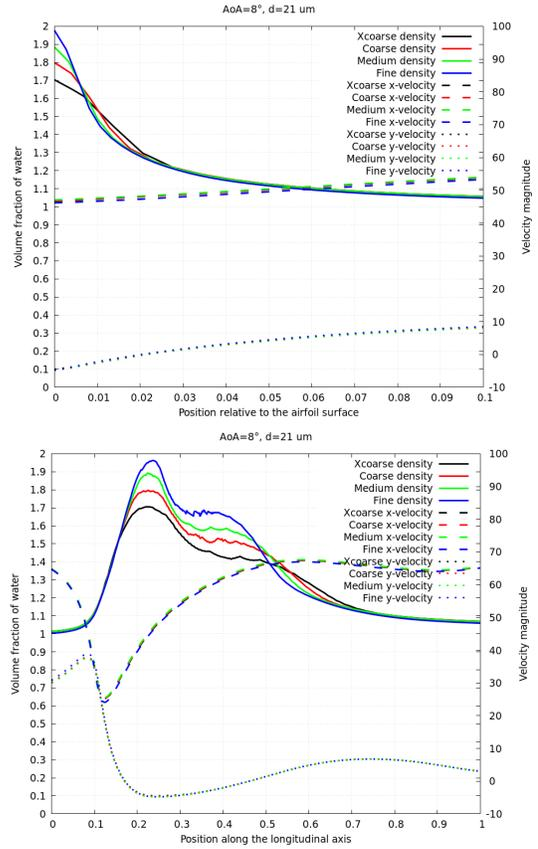
Figure 8: Normal and tangential volume fraction of water and velocity on the NACA 65<sub>2</sub>415 airfoil,  $d = 21 \mu\text{m}$ , Mach=0.23, AoA=0 = 8°, chord=0.928m
