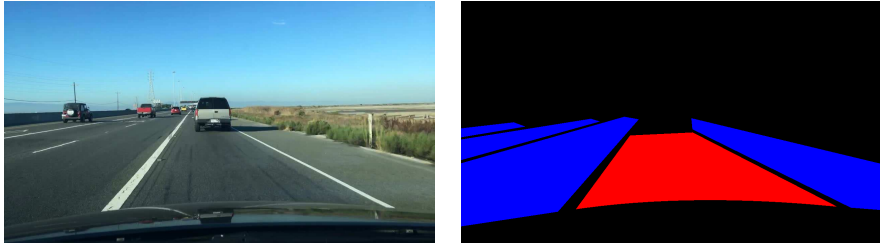
Fig. 1. A Sample Example of Annotation for Driveable Area Detection in BDD Dataset
