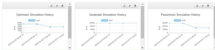
Fig. 5. shows a representation of KPIs including: (a) actual scaffold costs as well as (b) optimistic, (c) moderate and (d) pessimistic scenarios of the simulated duration
