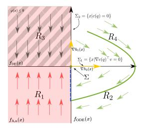
Fig. 2. Illustration of a phase plot of the time-frezing PSS from Definition 6. The red shaded area is the infeasible region of the CLS, where the trajectories of the auxiliary and DAE-forming dynamics flow. The green (solid) curve shows the resulting trajectory (a solution of the CLS) after discarding the time-frozen parts, cf. Theorem 10. The blue (dashed) curve shows a solution of the auxiliary ODE from Definition 5
